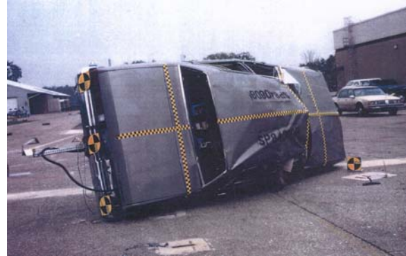
Figure 9. Malibu I Test 4 vehicle at rest with residual front seat intrusion and tenting.
