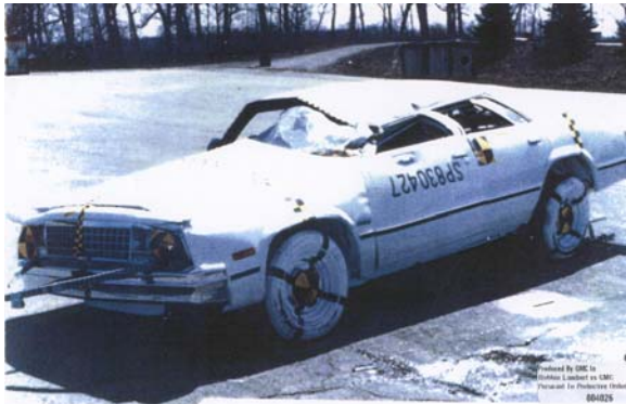
Figure 8. Malibu I Test 1 vehicle at rest with residual driver side intrusion.
