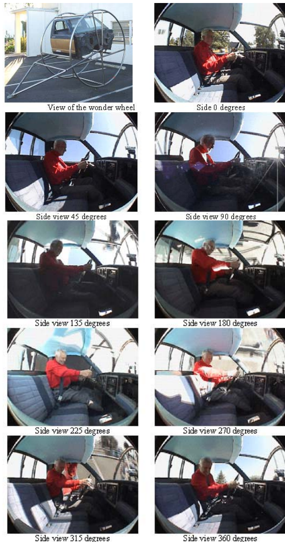
Figure 28. A human volunteer wearing a seat belt in the “Wonder Wheel”[6] that is rolling through 360 degrees. The occupant of this rotating fixture does not experience diving into the roof because his motion is essentially circular so that when the occupant’s head is nearest to the ground, it is traveling parallel to the ground.
